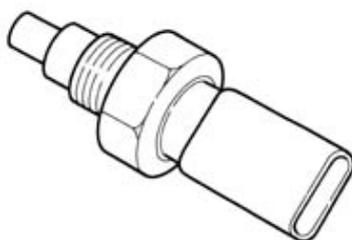
The sensor is constructed using semiconductor technology; therefore if the temperature of the sensor increases as the temperature of the coolant increases, the resistive value decreases.
