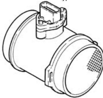
The intake air temperature sensor is built into the flow meter.
